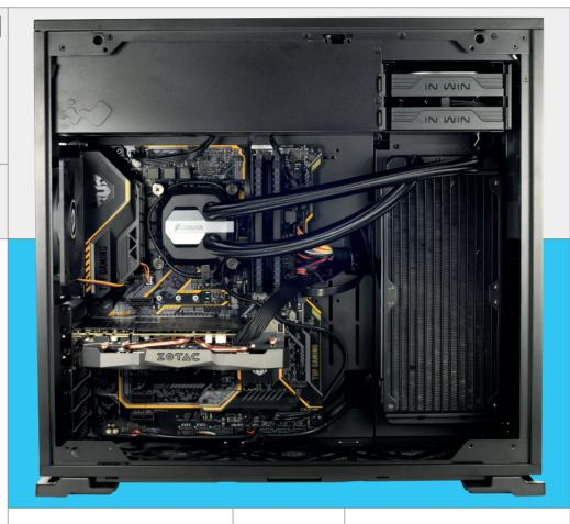
overclock that takes the base speed up to 1,620MHz. This isn't the fastest card around, but given the might of the Nvidia GTX 1080 GPU even at stock speeds, you can still expect awesome levels of 3D performance, with the potential to push things further through overclocking utilities.
